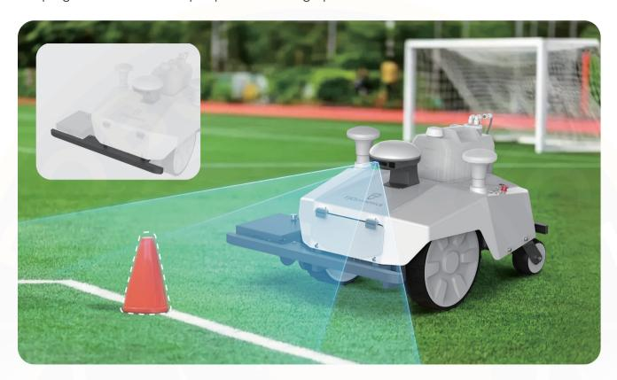
Come with a binocular camera for enabling automatic stop upon object detection during marking, delivering consistent performance even at nighttime.
